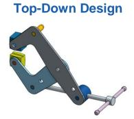
**Top-Down Design** is when the shape of an overall product is sketched first, and then different regions of that sketch are used to create the lower level parts and their features. Top-Down is a more intuitive way to approach a design because typically we, as designers, envision the final product first, then as time goes on, we refine the concept into finer and finer detail.
