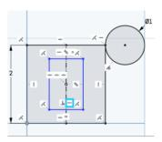
Enough dimensions and constraints will **fully-define** a sketch, changing the color of the sketch from blue to black. Dimensions refer to the distance and angle values of sketch entities. Constraints refer to the geometric relationships and rules within a sketch, common ones being Coincident, Horizontal, Vertical, Concentric, Midpoint, and Tangent.
